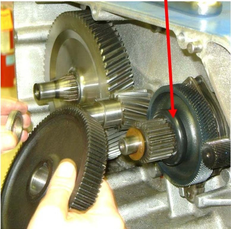
Load Brake Assembly has a Steel Thrust Washer behind it for wear
